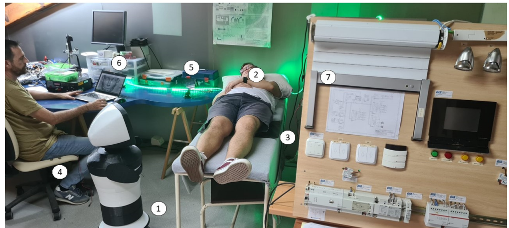
Figure 20. “Start of the day” test scenario: (1) Echo robot: 3D-printed Turtlebot base with Echo 8 and Alexa on head; (2) subject wearing the Empatica E4; (3) presence detector in bed; (4) presence detector in chair; (5) AAL user interface; (6) simulation of attention-status detection when viewing TV; (7) simulator of other home automation elements.
