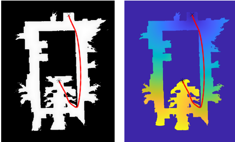
Figure 1. From left to right: initial binary map, time of arrival of the propagating wavefront T(x) . The path obtained with FMM is shown as a red line.
