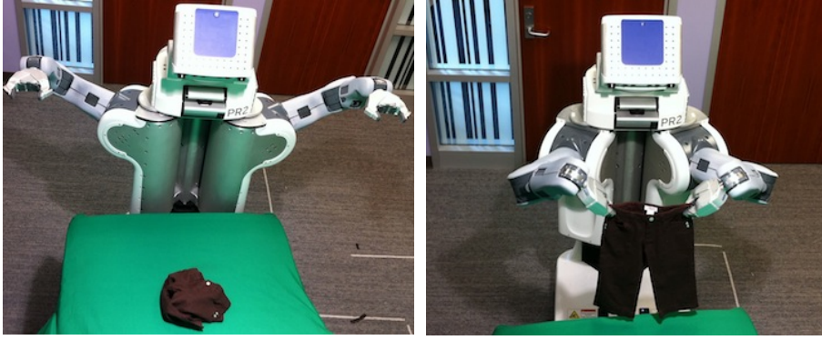
Figure 2.12: PR2 robot performing a folding sequence using the method presented in [7]. On the left, the initial crumpled state is shown. Through a sequence of manipulations the robot is able to unfold the pants to a known state (shown on the right), and the robot can then proceed to fold them. The figure was originally published as Figures 1 and 2 of “Bringing Clothing into Desired Configurations with Limited Perception” by Cusumano-Towner et al., Proc. IEEE ICRA 2011 © IEEE, 2011.
