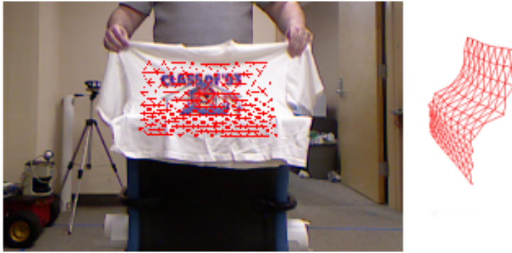
Figure 2.9: Performing state estimation on a deformable object from a video sequence [98]. On the left, the estimated garment state is superimposed to the source video frame. On the right, the same estimation is shown from a 45° angle. The figure was originally published as Figure 6d of “An Energy Minimization Approach to 3D Non-Rigid Deformable Surface Estimation Using RGBD Data” by Willimon et al., Proc. IEEE IROS 2012 © IEEE, 2012.
