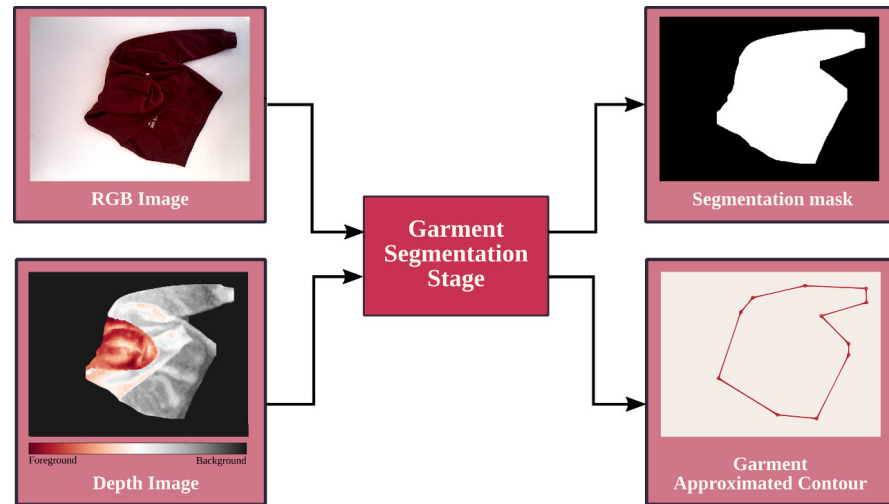
Figure 4.3: Garment Segmentation Stage using an RGB-D image, shown as an RGB and a depth image, as input.
