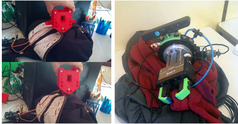
Figure 4.9: Grippers for the unfolding task. On the left, the gripper to be installed in the humanoid robot is depicted performing a grasping test. On the right, the custom gripper to be installed in the industrial robot is shown.
