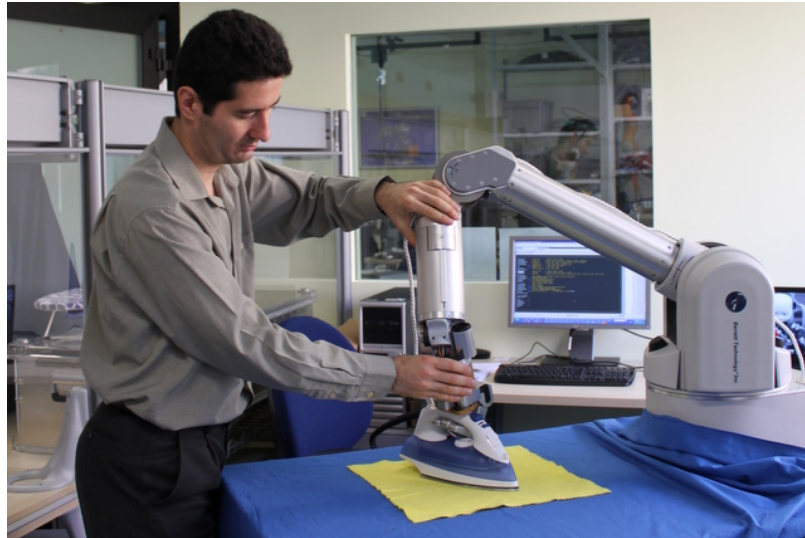
Figure 2.6: Kinesthetic teaching of the positional profile for the ironing task, introduced in [45]. The figure was originally published as Figure 8a of “Imitation Learning of Positional and Force Skills Demonstrated via Kinesthetic Teaching and Haptic Input” by Kormushev et al., Advanced Robotics © Taylor & Francis, 2011.
