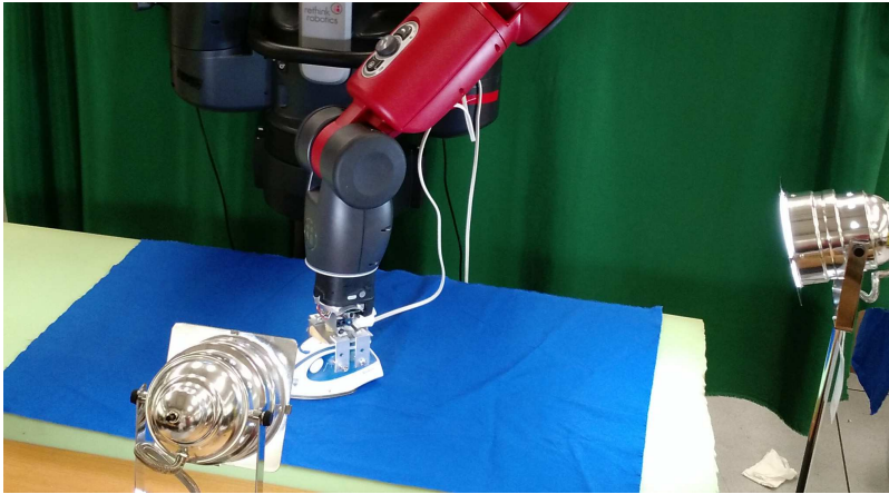
Figure 2.7: Experimental setup of the ironing method presented in [52], including the set of external lamps required for the curvature scan and the green foam required for passive compliance. The figure was originally published as Figure 8a of “Multi-Sensor Surface Analysis for Robotic Ironing” by Li et al., Proc. IEEE ICRA 2016 © IEEE, 2016.
