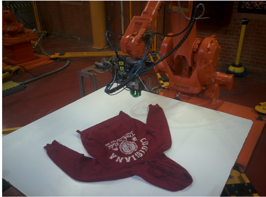
Figure 7.7: Unfolding setup for the industrial manipulator robot. The robot is equipped with a custom tool composed of a 3D printed gripper and an RGB-D camera. Garments are placed and folded on a white surface located in front of the robot.
