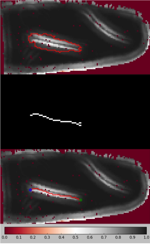
Figure 6: Different steps of the ironing path extraction from the WiLD 2D image. The largest wrinkled region is first selected (top). For this particular example, the leftmost wrinkle spanned \sim 3000 px and the rightmost one \sim 2000 px. The selected region is then skeletonized (middle), and from this skeleton the most suitable ironing path is computed (bottom). The two points, blue and green, represent the start and end points of the ironing path, respectively.
