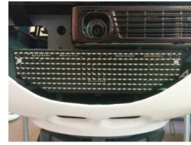
Figure 2. Detailed view of the hardware of an MBot’s matrix of LEDs.
