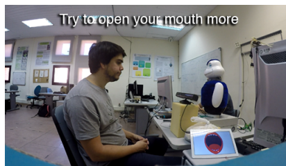
(d) If the mouth pose detected does not match the desired one, the robot corrects the user using voice and gestures while the tablet shows the target pose.
