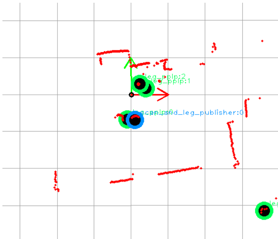
Figure 4.9: A capture of the benchmark of the leg detector PeoplePoseList Publisher . The arrows correspond to the position of the robot (the origin of the coordinates frame). In red, the current laser scan. In blue, the ground truth position of the user. In green, the users detections: four detections are visible, the one in the middle being a true positive and the three remaining false positives.
