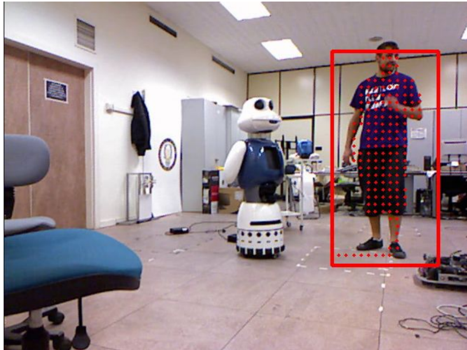
Figure 3.10: A sample true positive detection with the HOG PPLP. The red rectangle corresponds to the classical HOG detector. The red dots correspond to the 2D reprojection of the main 3D cluster.
