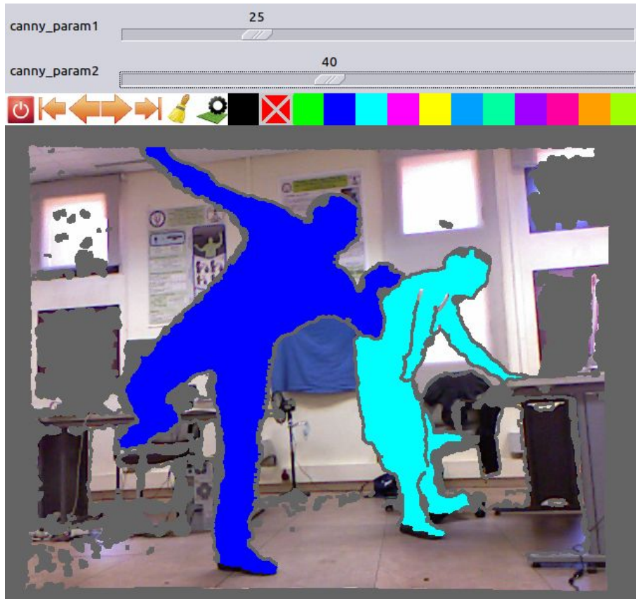
Figure 7.10: A sample view of the Graphical User Interface we developed for annotating images, called user_image_annotator .
