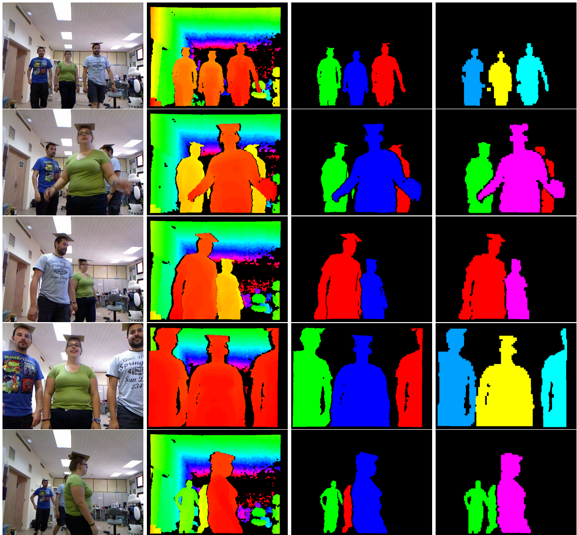
Figure 7.11: Some samples of the RLPD dataset. From left to right: column 1: the RGB image, column 2: the depth image; column 3: the manually labeled user map; column 4: the Kinect API NiTE user map. The dataset gathers some challenging features: partial (second row) or complete occlusions (third row), user not fully visible (fourth row). Note how the manual color indexing of the users is consistent (third column): the same user always corresponds to the same color. On the other hand, the NiTE algorithm performs swaps and create new users, or even merges users (fifth row).
