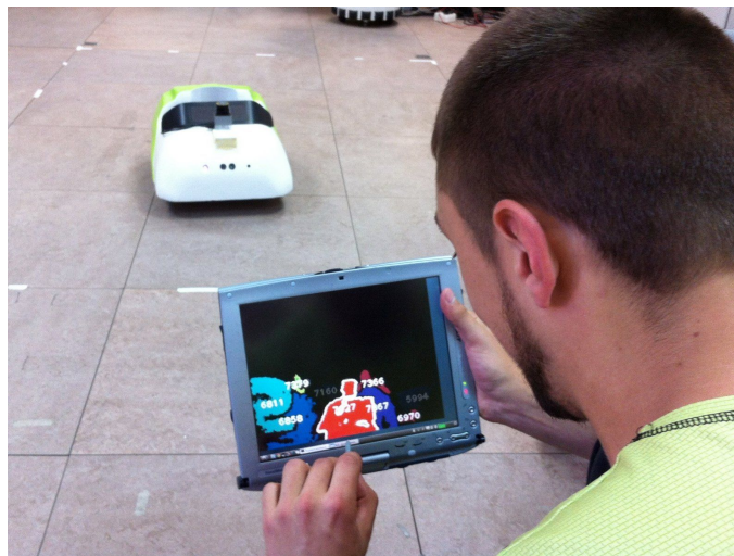
Figure 7.19: A sample picture of a user selecting the object-of-interest. It is indicated by the shape with a white border. The other objects are drawn with a different color.
