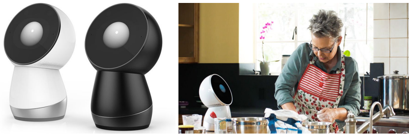
Figure 2.15: The social robot "Jibo". A user case is visible on the right, where Jibo is helping a user with her hands busy thanks to speech recognition. Images from http://www.myjibo.com/ .
