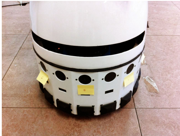
Figure 4.6: The microphones situated in the base of Maggie.
