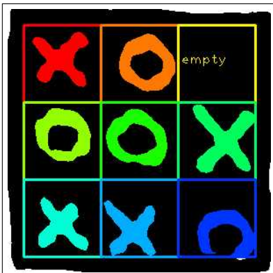
(c) Results of the image analysis by the tic-tac-toe algorithm
