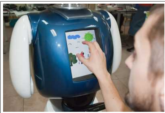
Fig. 3 An user interacting with Maggie through the touch screen in her chest. Here, he is using a very simple drawing application.
