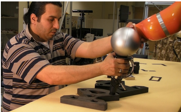
Fig. 2 Kinesthetic guiding using Kuka LWR arm in gravity compensation mode.
