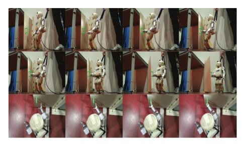
**Figure 4.10:** Snapshots of the humanoid robot performing the task of opening a door from different views.
