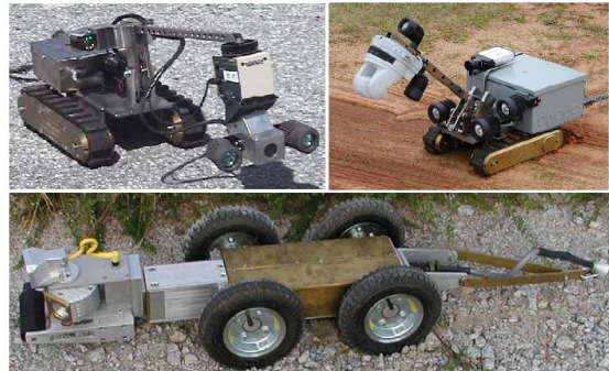
Figure 13. Three ventilation tunnel robotic inspection systems [63]
