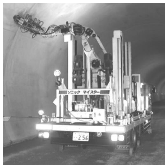
Figure 5. A robotic tunnel inspection system that uses the impact sound method [48]
