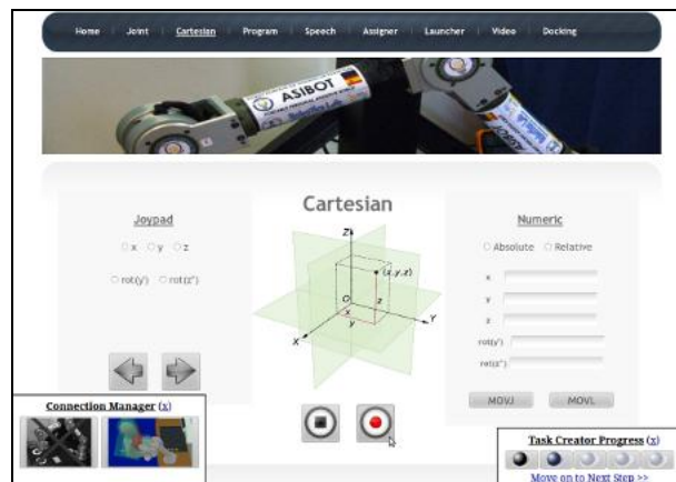
Figure 9. Points may be captured even when the robot is in movement
