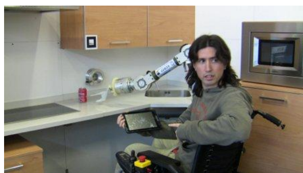
Figure 1. A developer explaining how to use the ASIBOT multi-modal interfaces
