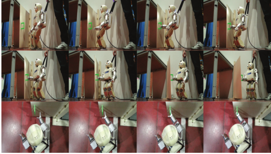
Figure 4.10: Snapshots of the humanoid robot performing the task of opening a door from different views.
