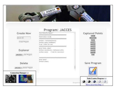
Figure 6. The robot Web Browsable interface Program Tab
