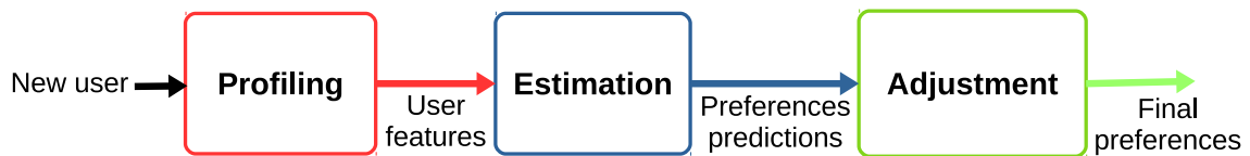
Figure 9.1: Our proposed Preference Learning (PL) System. It consists of three stages: user profiling, estimating their preferences, and adjusting the initial estimation using the interaction.
