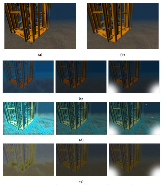
**Figure 6.** Processing of the simulator image for different sea models. (a) Original image from the UUV Simulator. (b) Forward-scattered image. (c) Atlantic ocean style, (e) Mediterranean sea style and (d) Muddy water style, with (from left to right) superposition value  $\alpha = 1$ ,  $\alpha = 0.4$  and with addition of two light sources.
