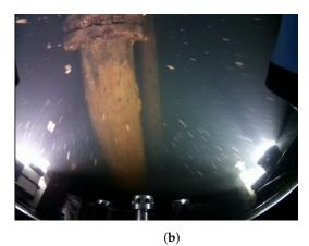
**Figure 1.** Deployment of the STAMS project underwater robot. (a) The modified version of the BlueROV2. (b) Capture obtained by the BlueROV2 camera in a flooded mine shaft during one of the STAMS field trials.
