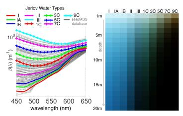
**Figure 3.** Left: Jerlov water types based on the attenuation coefficients  $\beta(\lambda)$ . Types I-III are oceanic waters, while those suffixed with 'C' represent coastal waters with increasing turbidity from 1 to 9. Right: appearance of a white surface viewed from various depths in the different water types. Image courtesy of Akkaynak, D. et al. [14].
