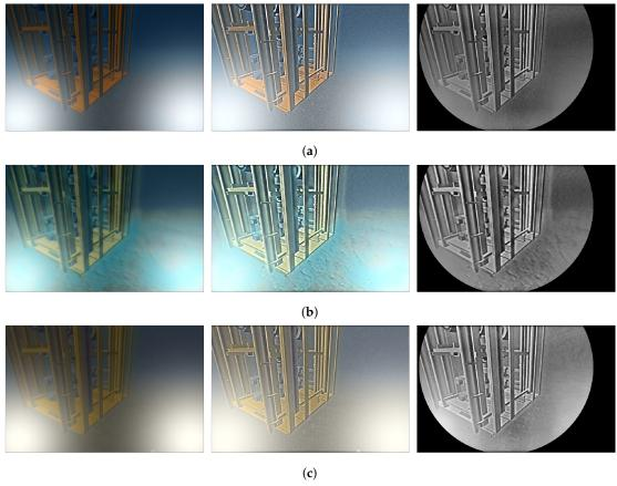
**Figure 8.** Image enhancement over the simulated underwater images for the (a) Atlantic Ocean, (b) Mediterranean sea, and for the (c) muddy water. From left to right: original image, homomorphic filtered image, and final result after applying the mask.
