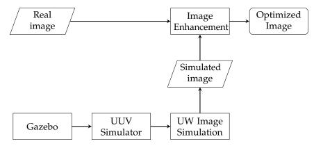
**Figure 2.** The proposed framework for simulation and development of underwater computer vision algorithms.
