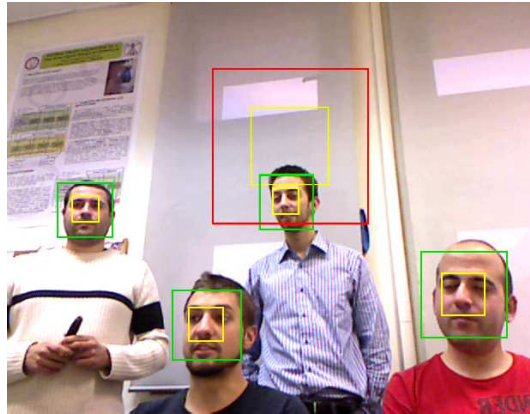
Figure 3: Results of the face detection algorithm on a sample image. The red and green rectangles correspond to the faces as detected by the Viola-Jones detector. The inner yellow boxes are the zones where the sample 2D points are being reprojected in 3D. The 3D-points bounding boxes of the correct detections pass the geometric constraints of a normal 3D face, hence their green color. The 3D-points bounding box of the wall is too big in dimensions and hence is discarded.
