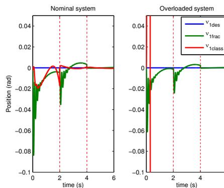
**Figure 5.7:** System response for joint 1 for the nominal (left) and overloaded (right) subsystem. In blue is the desired trajectory, in green the trajectory with the fractional order controller and in green the trajectory with the standard PID. In dotted red the limits of the three linearization regions.
