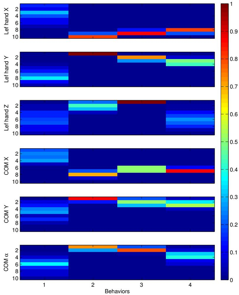
**Figure 4.8:** Behavior selector matrix. The columns represent the behaviors and the rows represent the substates in a state. For each substate the color represents the probability of being in a behavior.
