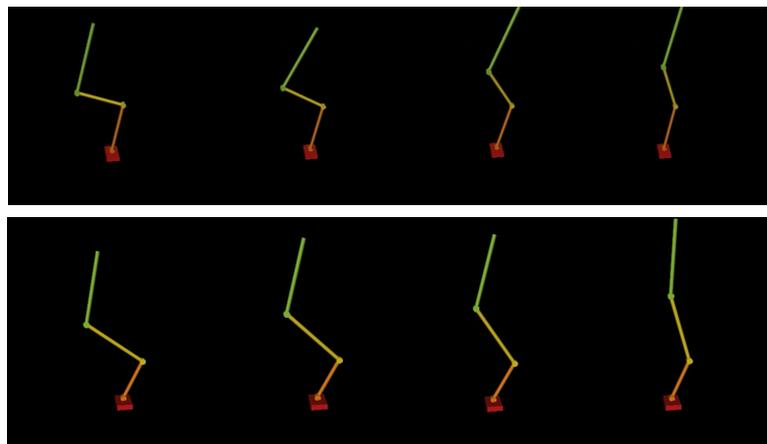
**Figure 3.12:** Several snapshots of an actuated 3-link kinematic chain simulating the movement of standing up. The upper part simulates the imitation behavior while the lower part simulates the innovation. In the imitation line it can be seen that the kinematic chain lean forward while in the innovation part the movement is straighter.
