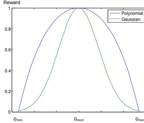
**Figure 3.7:** Two reward functions. The blue one is a polynomial function of 4th degree, the green one is a gaussian-like function whose maximum is one. The parameter  $\theta$  represent the ZMP or the torque of the actuated 3-link kinematic chain.
