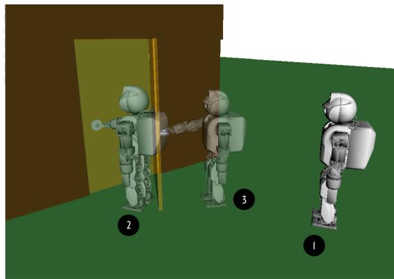
**Figure 4.1:** Behavior sequence detail of the high-level task of opening a door by a simulated HOAP-3 robot. The robot starts at point 1, it approaches to point 2 near the door in a way it can reach the knob, after grasping the door, it pulls back the door to point 3. Finally, it releases the knob.
