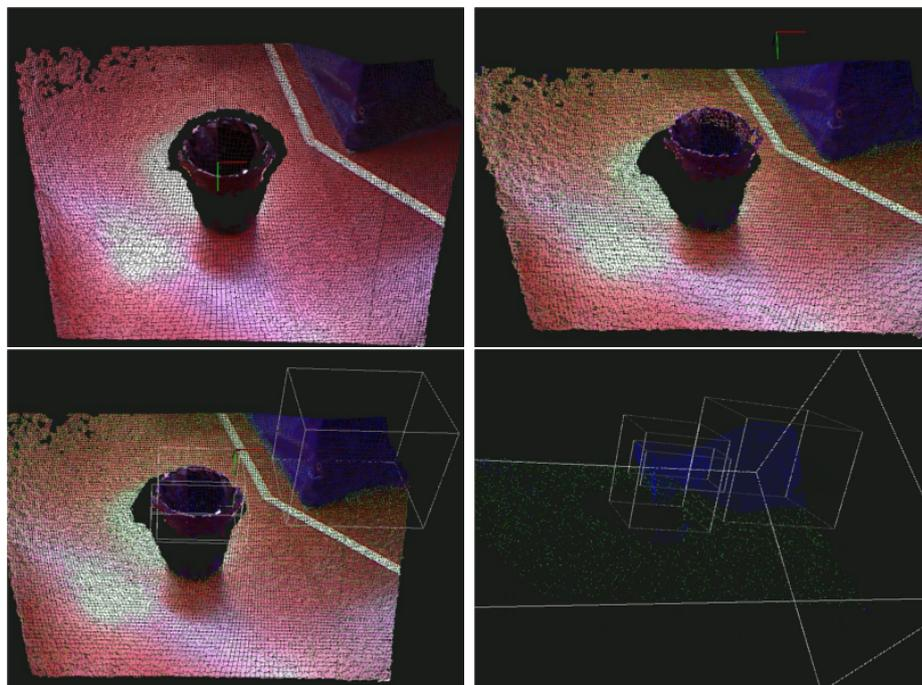
**Figure 6.7:** *In the snapshot the environment recognition is performed. The green dots represents the floor and the blue dots represent the obstacles. Finally a bounding box of the obstacles is extracted together with their dimensions and their positions.*
