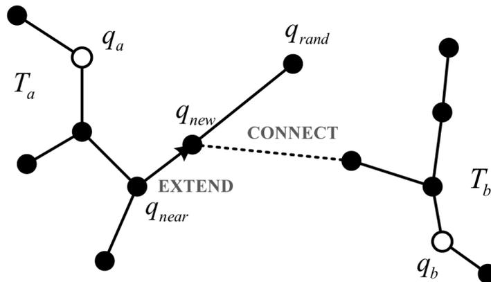
**Figure 6.3:** Process of RRT-Connect merging two RRT trees.
