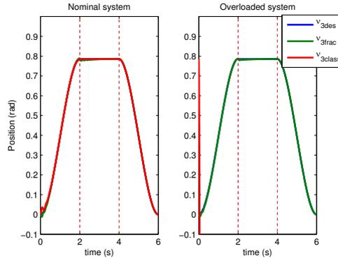
**Figure 5.9:** System response for joint 3 for the nominal (left) and overloaded (right) subsystem. In blue is the desired trajectory, in green the trajectory with the fractional order controller and in red the trajectory with the standard PID. In dotted red the limits of the three linearization regions.
