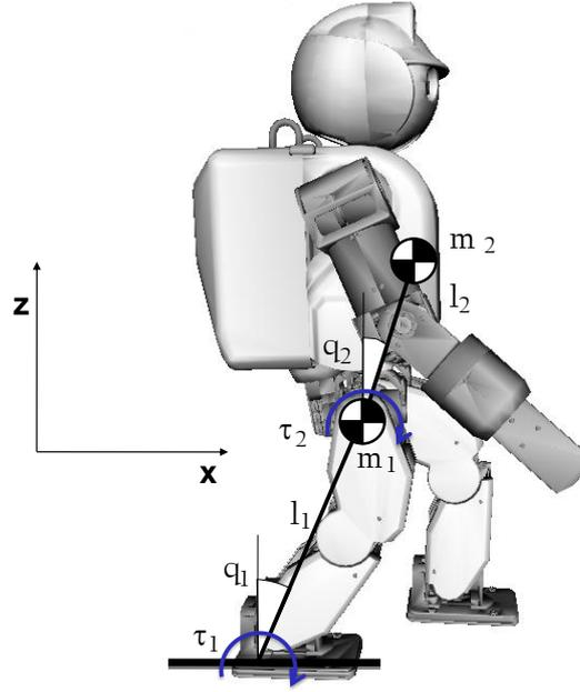
**Figure 2.2:** *Double inverted pendulum*
