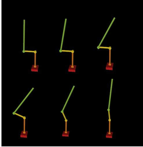
Figure 5.4: Simulation of triple inverted pendulum trajectory.
