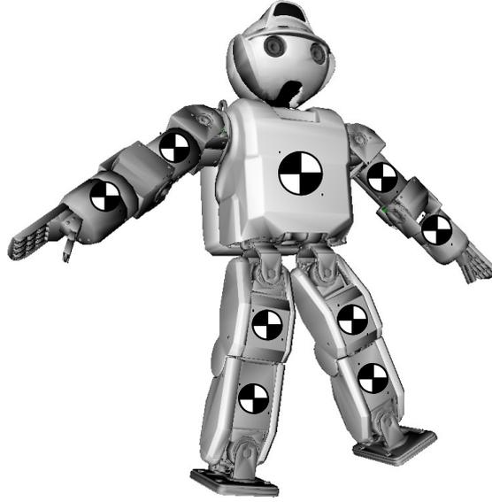
**Figure 2.4:** Snapshot of a distributed mass model of the humanoid HOAP-3.
