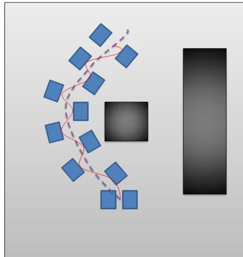
**Figure 6.5:** *Top-view schema of the complete scenario with obstacles in dark gray, global path planning represented by the dotted line, steps plotted as blue boxes and finally COM path shown with a red thin line.*
