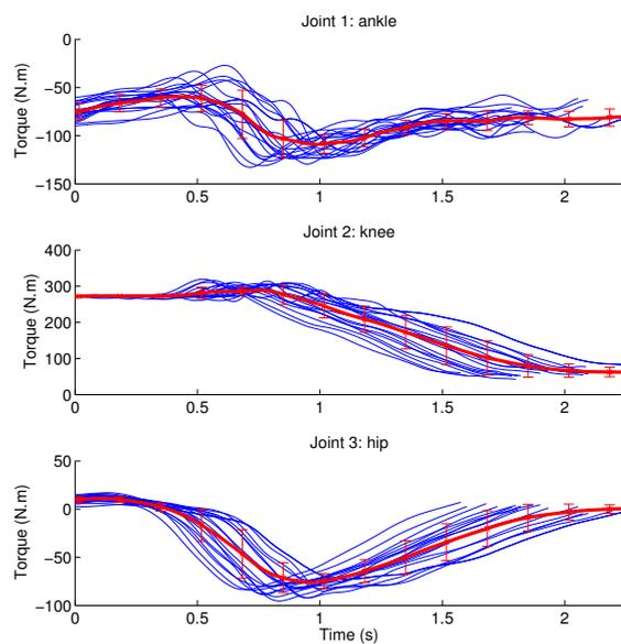
**Figure 3.6:** Actuated 3-link kinematic chain’s torques of the 20 demonstrations of one of the subjects standing up. The first joint of the 3-link kinematic chain corresponds to the human ankle, the second one to the knee and the third one to the hip. In red are the mean and standard deviation.
