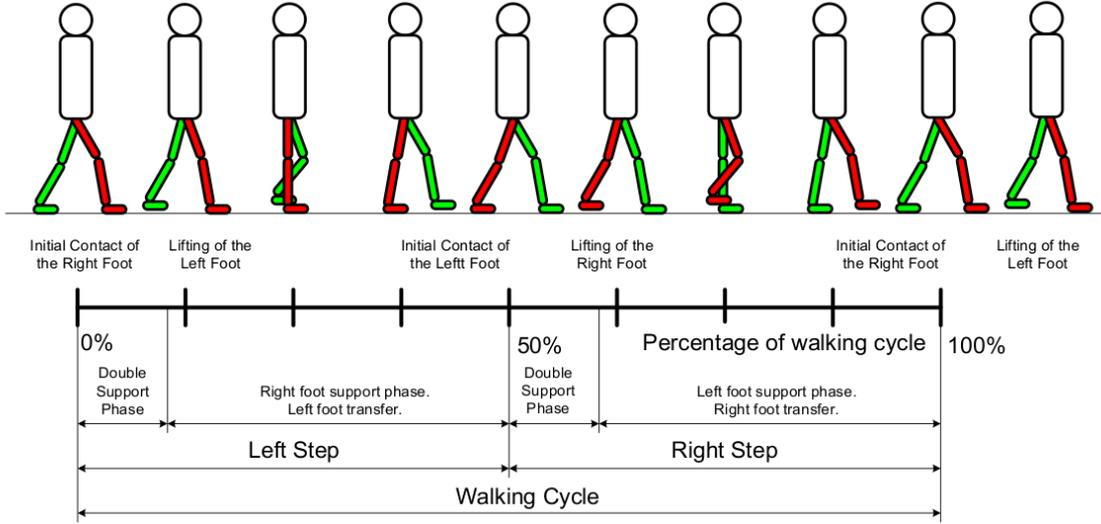
**Figure 2.6:** *Walking cycle phases* ©(Kaynov, 2008)
