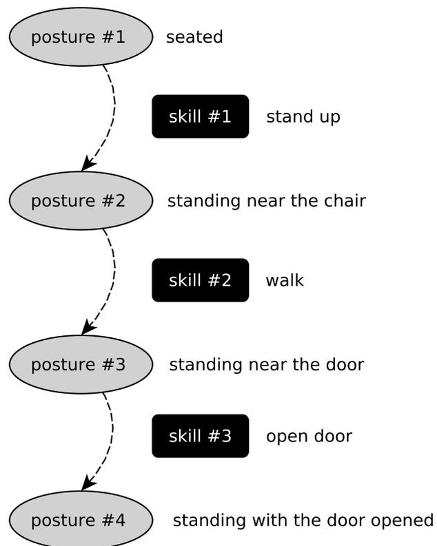
**Figure 6.9:** *Postural skill generation process for fulfilling the order “stand up from a chair, walk to the door and open it” in a humanoid robot. It consists on 4 postures, which are the initial and final states of the movement, and three skills, which corresponds to the dynamical transition between postural primitives.*
