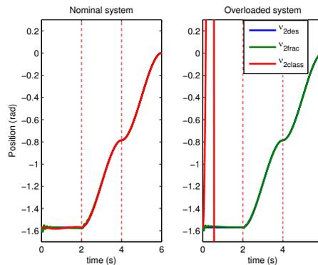
**Figure 5.8:** System response for joint 2 for the nominal (left) and overloaded (right) subsystem. In blue is the desired trajectory, in green the trajectory with the fractional order controller and in green the trajectory with the standard PID. In dotted red the limits of the three linearization regions.
