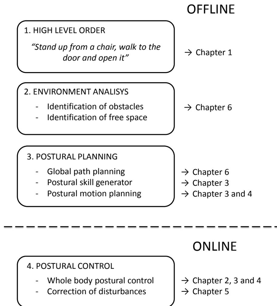
**Figure 6.1:** Complete proposed architecture for the humanoid behavior. It consists of four modules. The high level task, an environment analysis, an offline postural planning and an online postural control.
