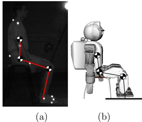
**Figure 3.2:** (a) Snapshot of the high frequency camera of the MOCAP system with a subject seated on a chair and markers on his body. Actuated 3-link kinematic chain is overlaid. (b) A simulation of the humanoid HOAP-3 seated on a chair and the 3-link kinematic chain.
