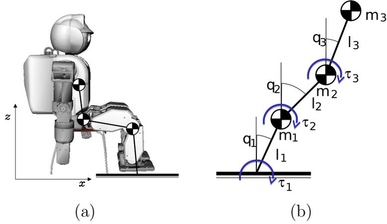
**Figure 2.3:** (a) Reduced model of HOAP humanoid robot seated on a chair. The proposed model is a two dimensional triple inverted pendulum with massless links and the center of mass at the tip of the pendulum. (b) Triple inverted pendulum with masses, lengths, torques and positions.
