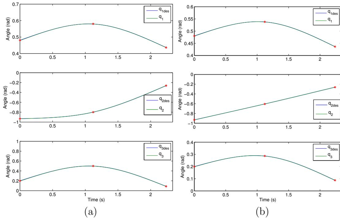
**Figure 6.4:** Desired joint trajectory of the three actuated joints and output of the PD controller in the imitation process (a) and in the innovation process (b) of a humanoid robot standing up from a chair. The red dot represents the initial, middle and final points of the piecewise polynomial of (4.24).
