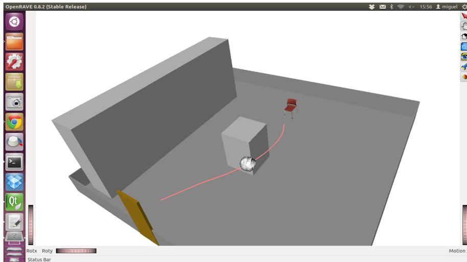
**Figure 6.8:** *Resulting path planning of the COM plotted in OpenRave. HOAP head represents the COM of the complete robot. It is also represented the obstacles as grey boxes.*
