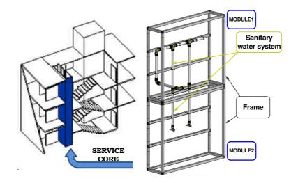
Figure 3 Service Core and 'wet area'
