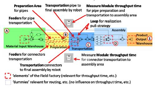
Figure 4 Field Factory Simulation model (Courtesy of Fraunhofer IAO & UC3M)
