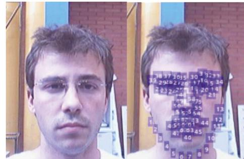
Fig. 20 Original face image on the left and the same image with landmarks of 63 characteristic points superposed on the right.
