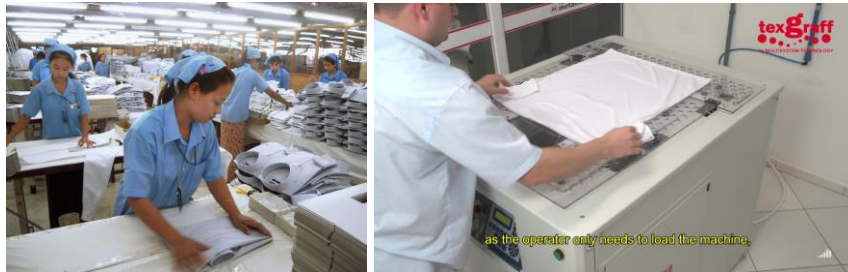
Fig. 1. Current clothes folding solutions available for garment folding. On the left, human workers folding clothes in a textile factory. On the right, an automated solution available in the market, manufactured by Texgraff©.
