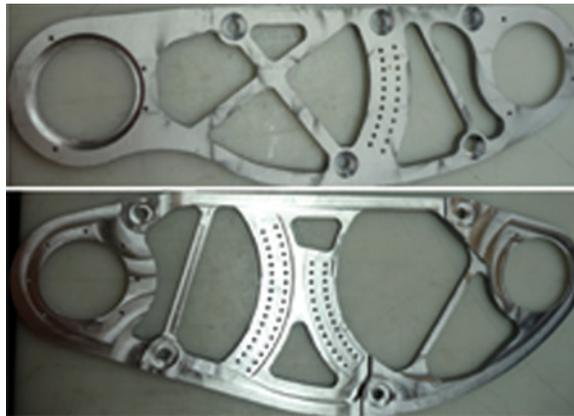
**FIGURE 12** Manufactured tibia (top) and thigh (bottom) (color figure available online).
