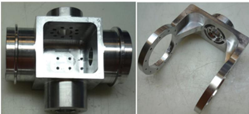
**FIGURE 14** Manufactured hip cross part (left) and hip fork part (right) (color figure available online).
