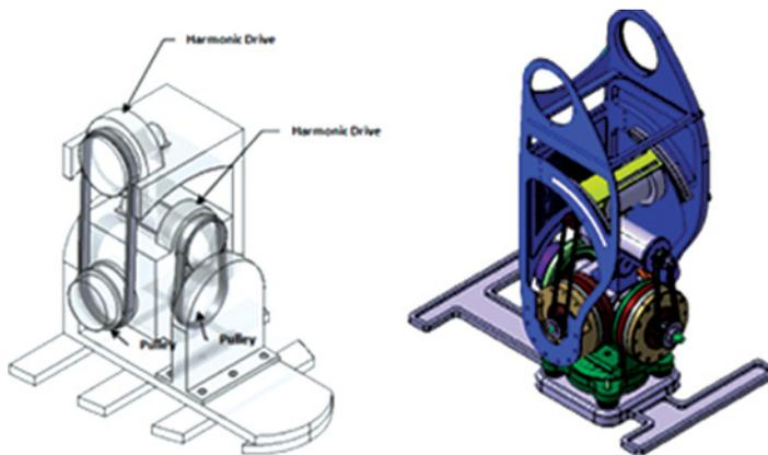
**FIGURE 5** Previous design of robot ankles (color figure available online).
