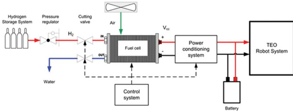
**FIGURE 15** Hybrid fuel cell simplified scheme (color figure available online).
