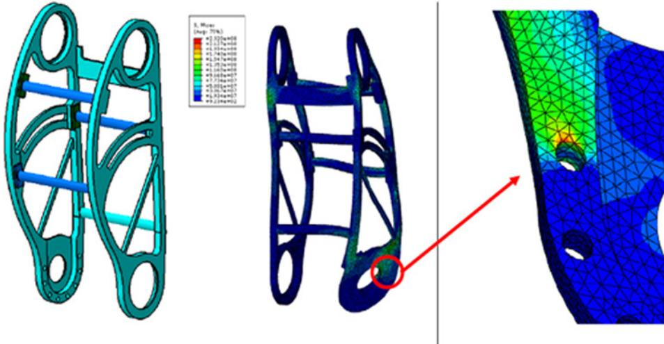
**FIGURE 11** Tibia model R24. Weight: 917 g; maximum Von Mises tension:  $2.32 \text{ e}^8 \text{ N/m}^2$  (color figure available online).
