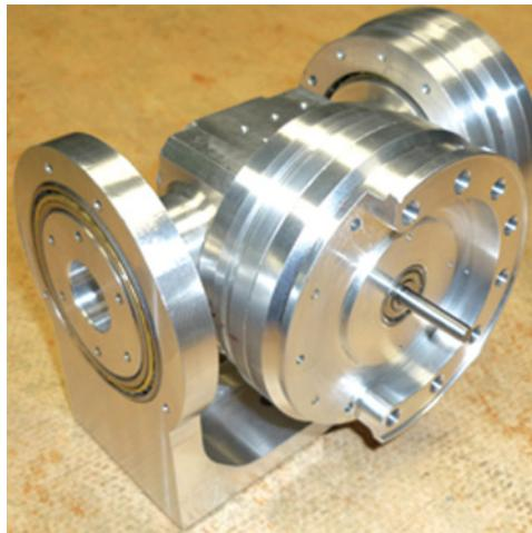
**FIGURE 10** Assembled ankle: cross and fork manufactured parts (color figure available online).
