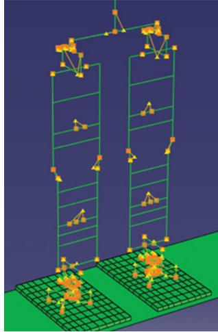
**FIGURE 3** Multibody model of the lower part of the humanoid robot TEO (color figure available online).
