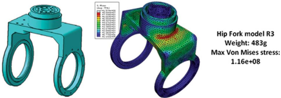
**FIGURE 13** Hip cross part model of the humanoid robot TEO (color figure available online).
