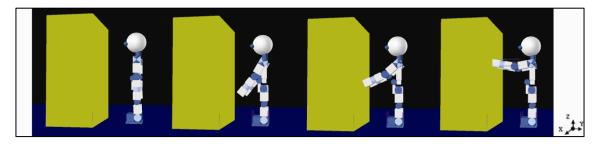
Fig. 15. Sequence of motions for HOAP-3 touching a wall.
