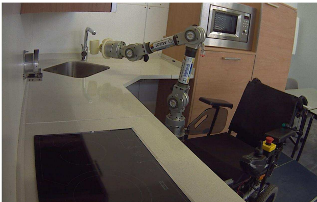
Figure 2. ASIBOT in Kitchen situated on Wheelchair DS
