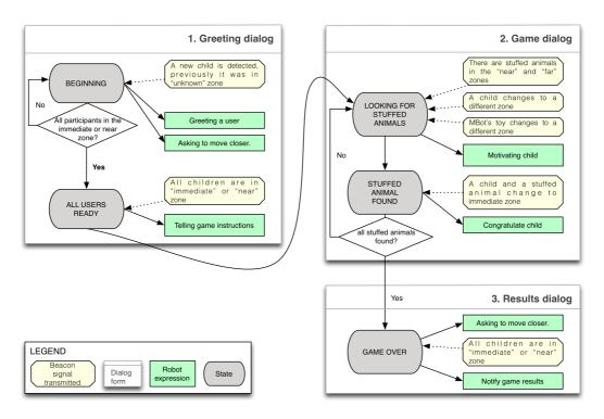
Fig. 5. Flow diagram of the dialogs in the hide-and-seek game. The information provided by the BLE beacons is detailed.
