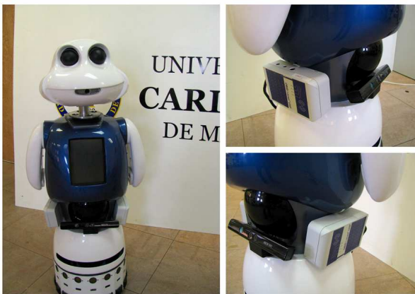
Fig. 6. The robot Maggie with the UHF antennae.
