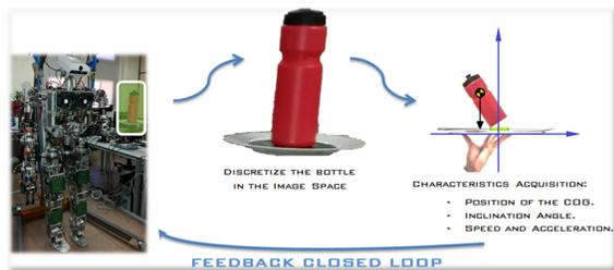
Figure 2: Steps followed to acquire the bottle characteristics and close the loop.
