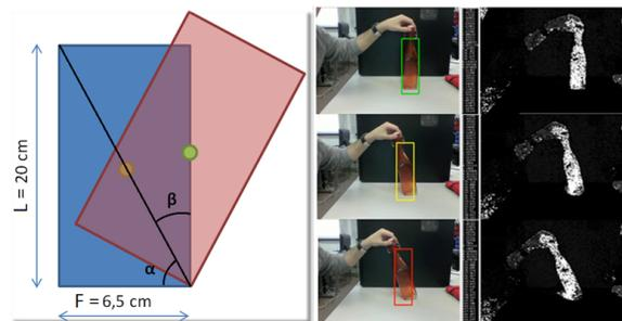
Figure 4: Tilt angle detected by computer vision techniques
