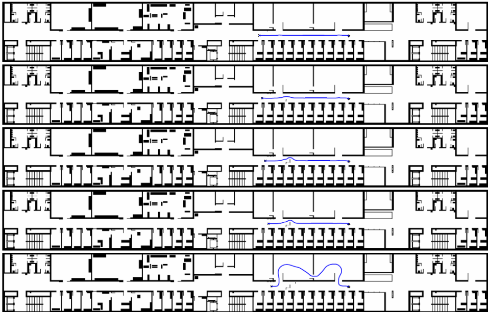
Fig. 12. Dynamical evolution of the path when the robot reads information about the new obstacles that are not in the previous map and the robot cannot pass through the corridor.
