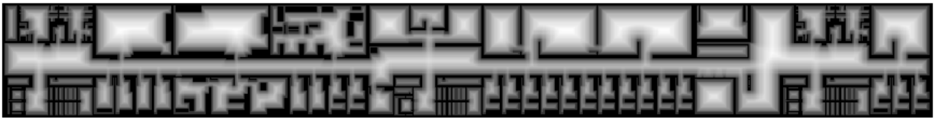
Fig. 9. Log of the Distance transform applied of the environment map of the Robotics Lab.
