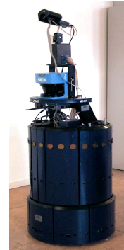
Figure 10. B21 robot with a laser telemeter
